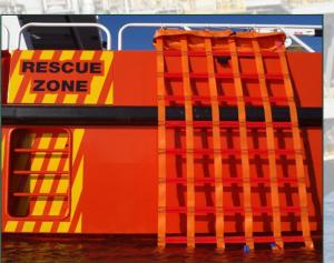
The Fibrelight Recovery Cradle is primarily designed for use by rescue craft, rigid inflatables and ship lifeboats and marinas, however it can have multiple other uses.
