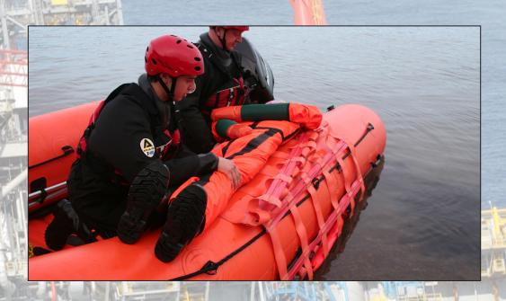
The Fibrelight Cradle can be used to bring incapable persons onboard. This is achieved through one end of the cradle being secured to the craft and the outboard end being held outwards by hand, boat hook or bridle. The incapable person is then guided into the cradle and the outboard end is hauled in rung by rung. The person is then safely rolled over the side and into the craft.
